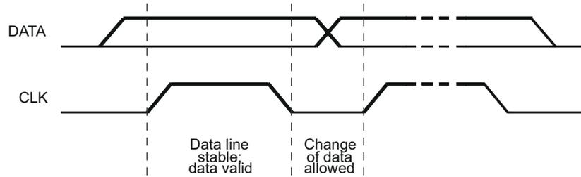
**Figure 8-3. Bit Transfer on the Serial Interface**
