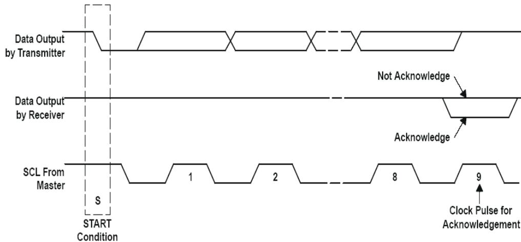
**Figure 8-4. Acknowledge on the I<sup>2</sup>C Bus**
