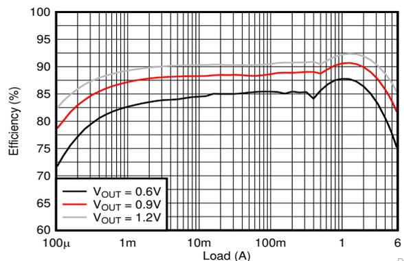
Efficiency at V<sub>IN</sub> = 3.3 V
