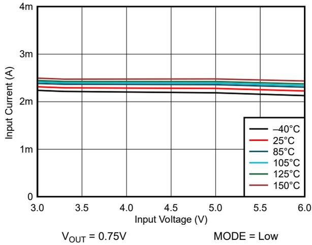
Figure 7-1. Operating Supply Current (Power Save Mode)
