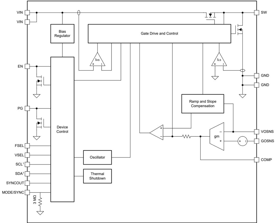
1. In device variants without I<sup>2</sup>C the SDA and SCL pins are internally connected, but their functionality is disabled.
