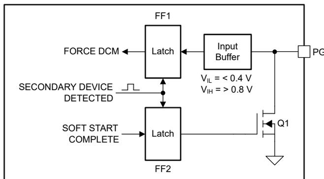
**Figure 8-13. Power-Good Functional Block Diagram (Secondary Device)**
