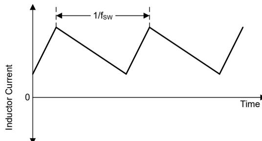
**Figure 8-2. Continuous Conduction Mode (PWM-CCM) Current Waveform**
