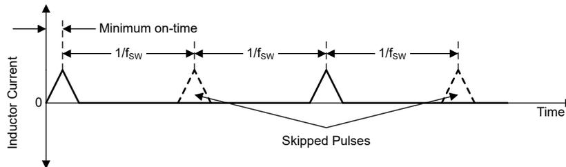
**Figure 8-4. Discontinuous Conduction Mode (PFM-DCM) Current Waveform**
