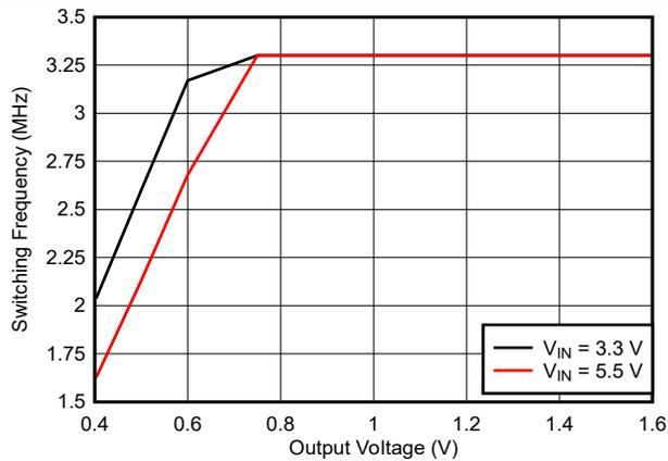
Figure 7-5. Maximum Switching Frequency vs  $V_{IN}$  and  $V_{OUT}$
