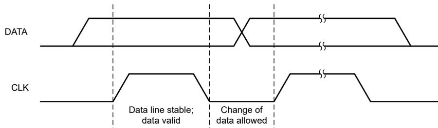
**Figure 8-16. Bit Transfer on the Serial Interface**
