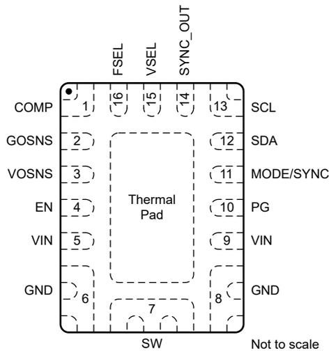
**Figure 6-1. 16-Pin RXS VQFN Package (Top View)**
