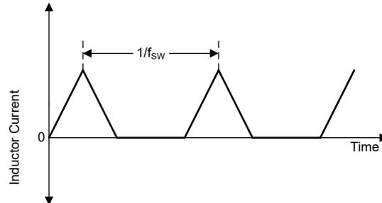
**Figure 8-3. Discontinuous Conduction Mode (PWM-DCM) Current Waveform**
