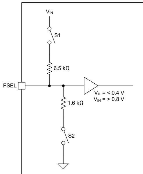
**Figure 8-10. FSEL R2D Converter Functional Block Diagram**
