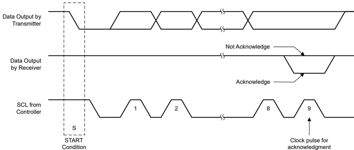
**Figure 8-17. Acknowledge on the I<sup>2</sup>C Bus**
