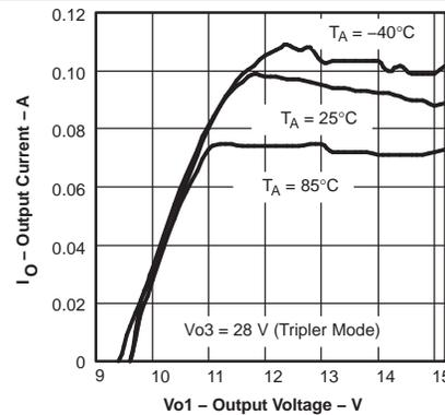
Figure 14. V<sub>O3</sub> Maximum Load Current (tripler mode)
