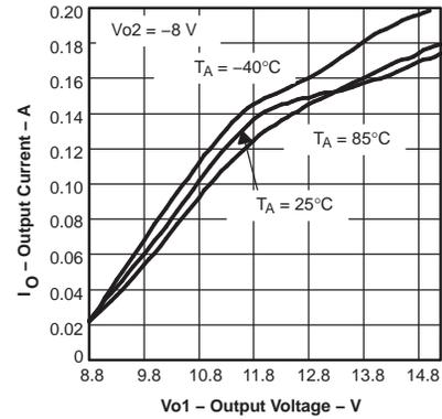
Figure 12. V<sub>O2</sub> Maximum Load Current
