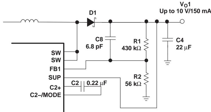
Figure 2. Feed-forward Capacitor
