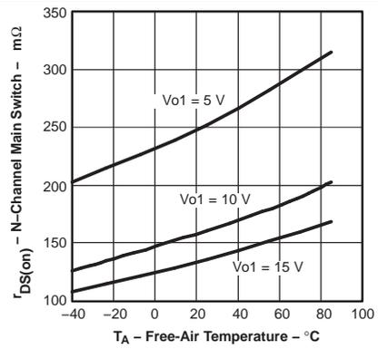
Figure 1.  $r_{DS(on)}$  N-Channel Main Switch vs Free-air Temperature
