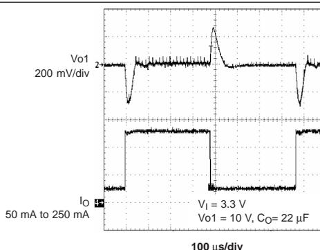
Figure 8. Load Transient Response  $1 \times C_O$
