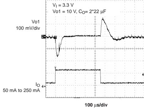
Figure 9. Load Transient Response 2 x C<sub>O</sub>
