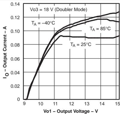
Figure 13. V<sub>O3</sub> Maximum Load Current (doubler mode)
