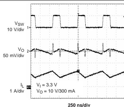
Figure 6. PWM Operation Continuous Mode
