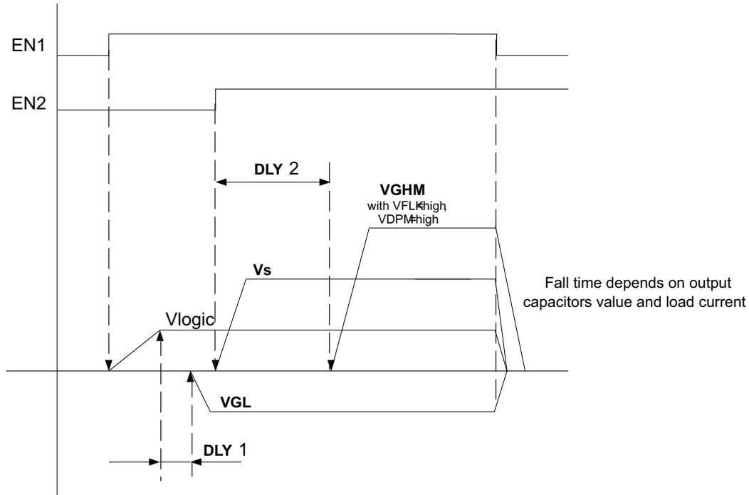
**Figure 20. Power-on Sequencing Using EN1 and EN2**
