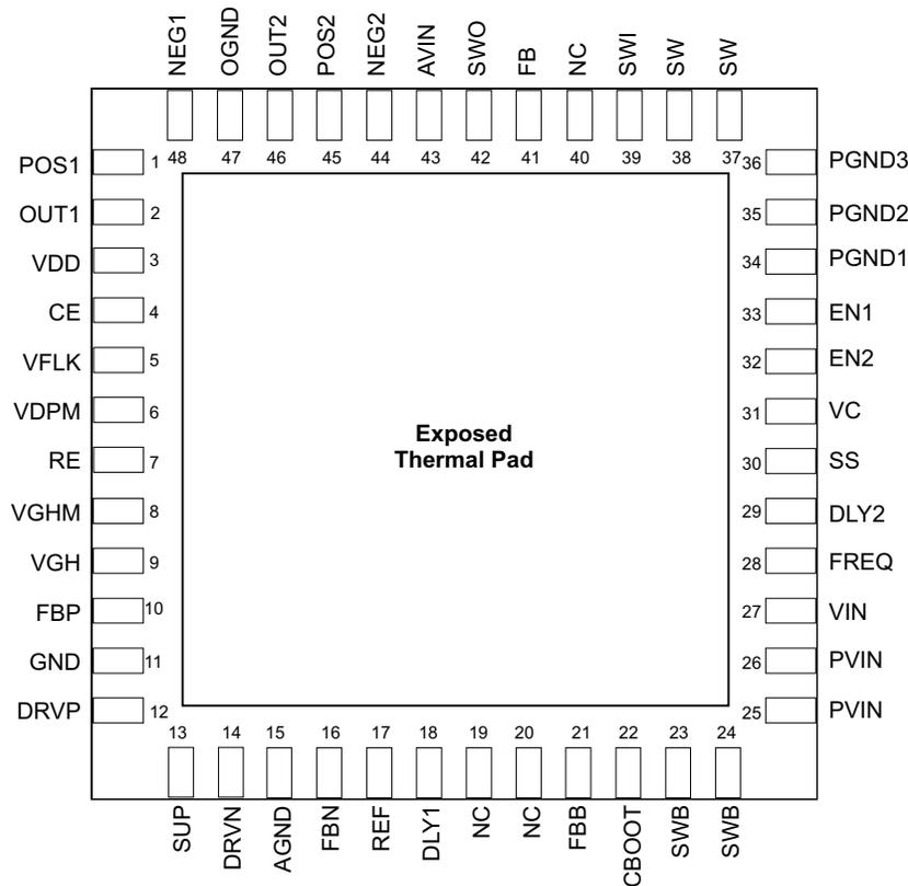
NOTE: The thermally-enhanced PowerPAD is connected to PGND1 (Device power Ground). NC pin is internally not connected.
