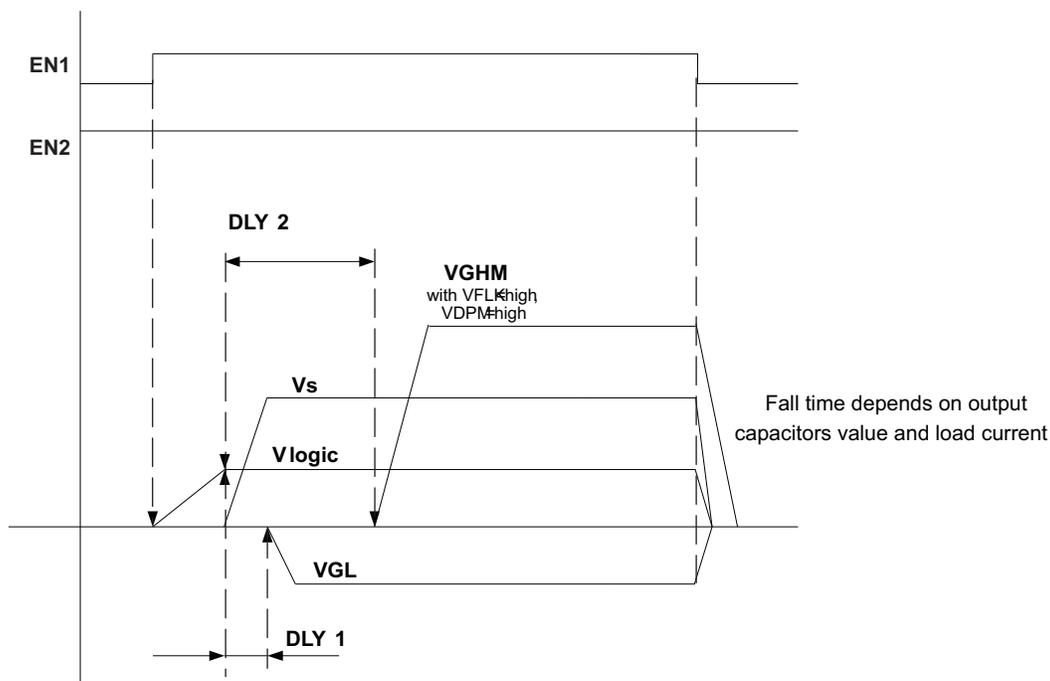
Figure 19. Power-On Sequencing With EN2 Always High (EN2=VIN)
