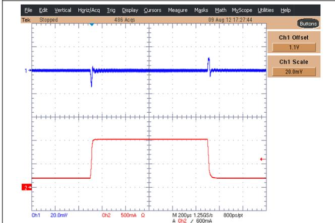
Figure 73. DCDCx Load Transient Response, 1.1  $V_{OUT}$ , 200-1000-200 mA Load
