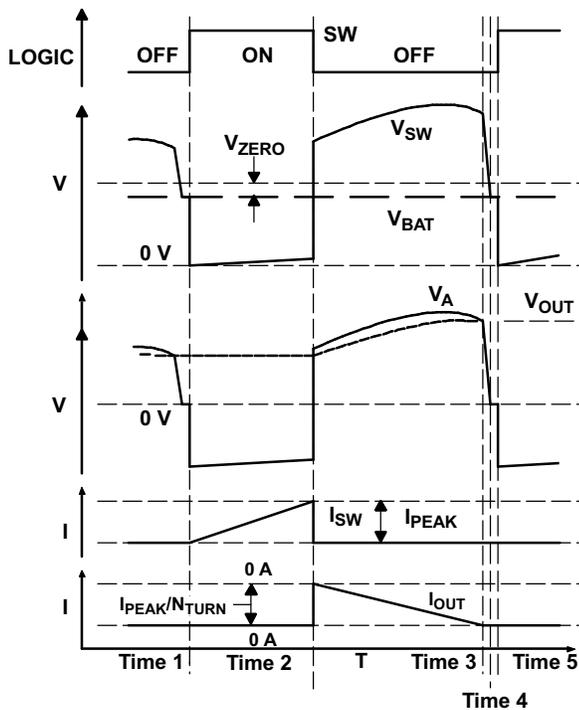
Figure 5. Timing Diagram at One Switching Cycle
