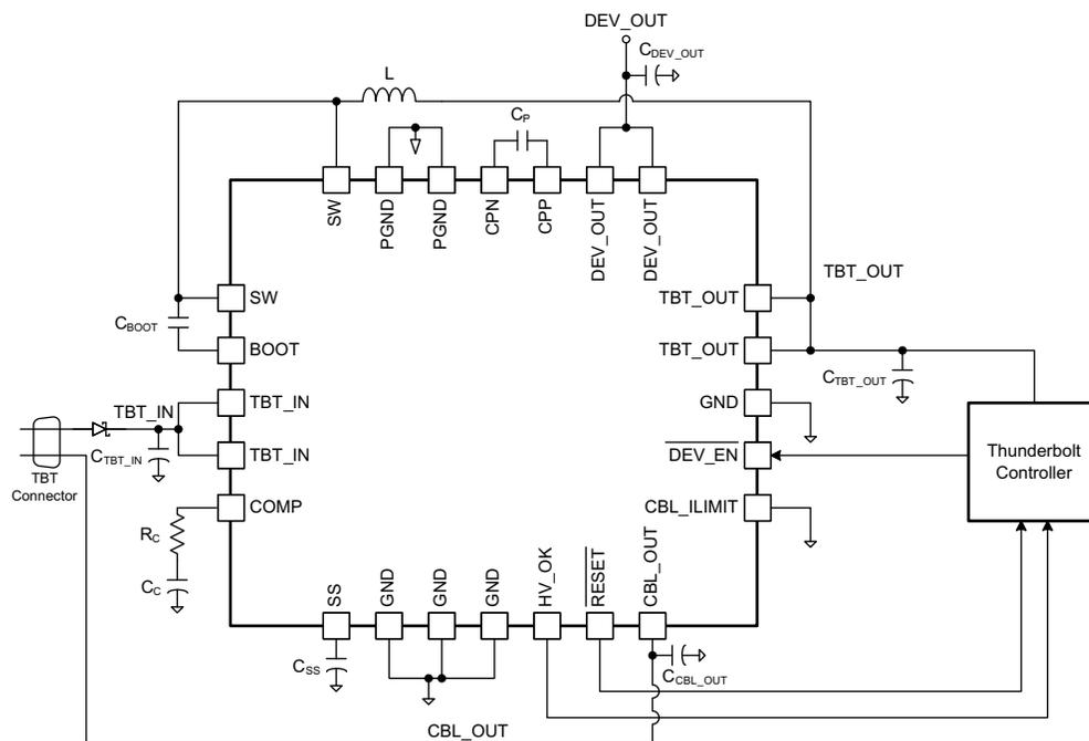
Figure 13. Typical Application (Single-Port Bus-Powered Thunderbolt™ Device)
