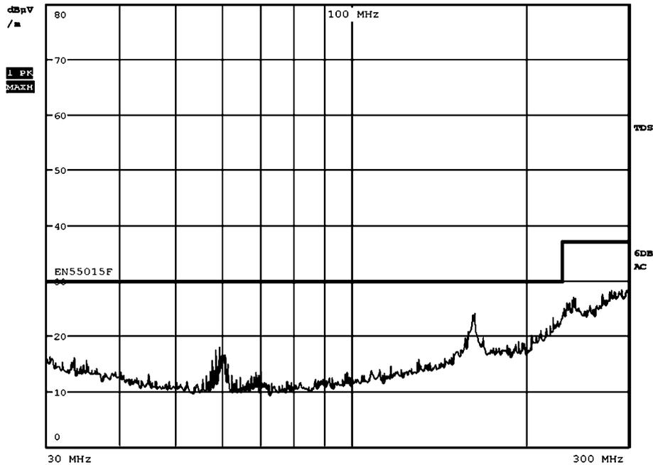
Figure 37. Complies with EN55015 Radiated Emissions (HORI. / HEIGHT=3.0m / RANGE=10m)
