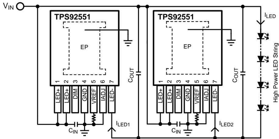
Figure 34. Parallel Operation Circuit Schematic for  $I_{LED} = 900\text{mA}$
