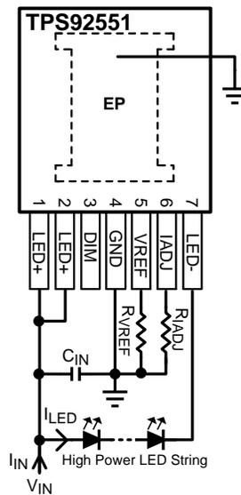
**Figure 32. TPS92551 Application Schematic for  $I_{LED}$  Setting**
