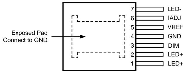
Figure 5. 7-Pin PFM (Top View)
