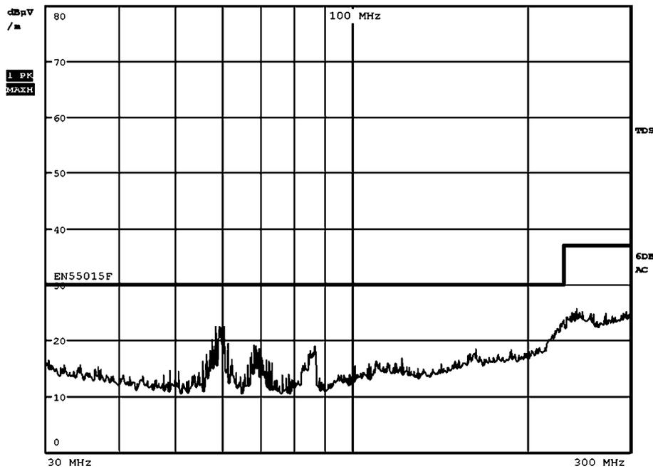
Figure 38. Complies with EN55015 Radiated Emissions (VERT. / HEIGHT=1.0m / RANGE=10m)
