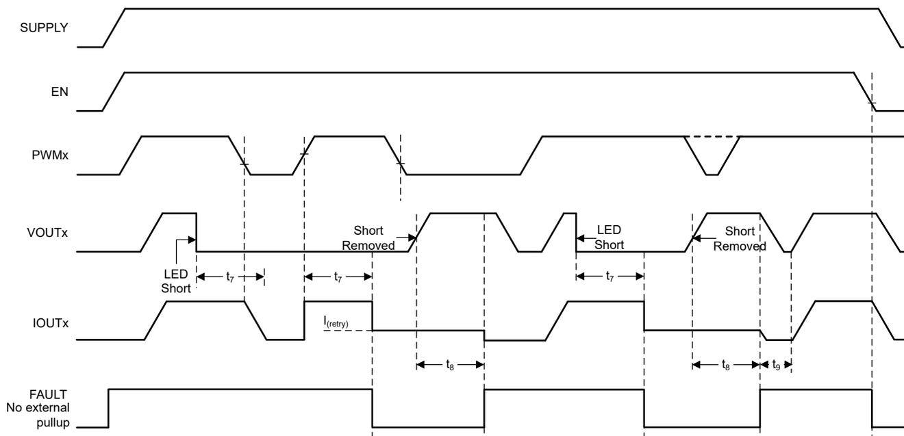
**Figure 6-3. LED Short-to-GND Detection and Recovery Timing Diagram**
