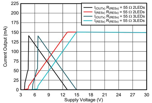
Figure 5-8. Output Current Distribution vs Supply Voltage
