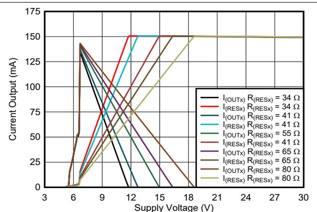
Figure 5-6. Output Current Distribution vs Supply Voltage
