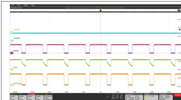
Ch1 =  $V_{(SUPPLY)}$     Ch2 =  $V_{(DIAGEN)}$     Ch3 =  $V_{(PWM1)}$
