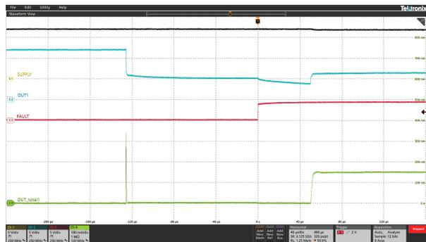
Ch1 =  $V_{(SUPPLY)}$     Ch2 =  $V_{(OUT1)}$     Ch3 =  $V_{(FAULT)}$
