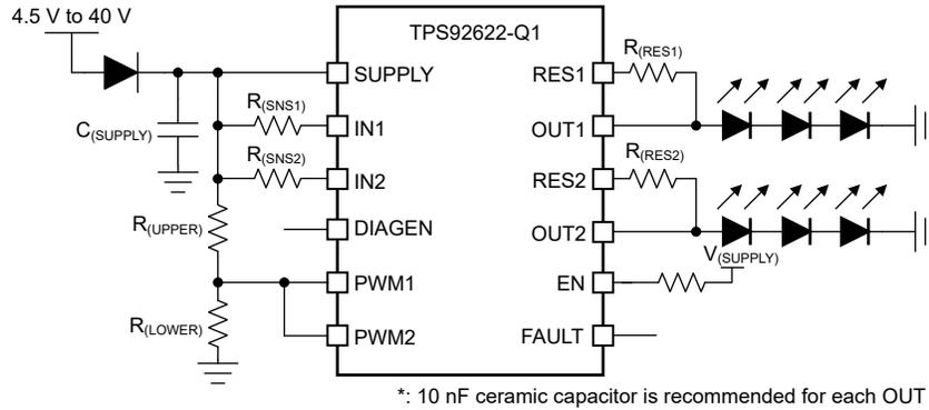
Figure 6-2. Application Schematic for Supply Control LED Brightness
