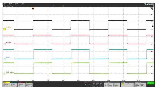
Ch1 =  $V_{(SUPPLY)}$  Ch2 =  $V_{(OUT1)}$  Ch3 =  $V_{(PWM1)}$
