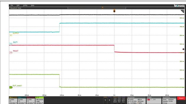
Ch1 =  $V_{(SUPPLY)}$     Ch2 =  $V_{(OUT1)}$     Ch3 =  $V_{(FAULT)}$
