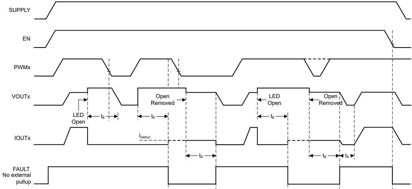
Figure 6-4. LED Open-Circuit Detection and Recovery Timing Diagram
