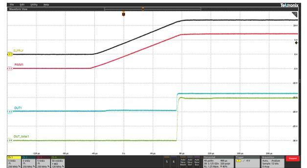
Ch1 =  $V_{(SUPPLY)}$  Ch2 =  $V_{(OUT1)}$  Ch3 =  $V_{(PWM1)}$
