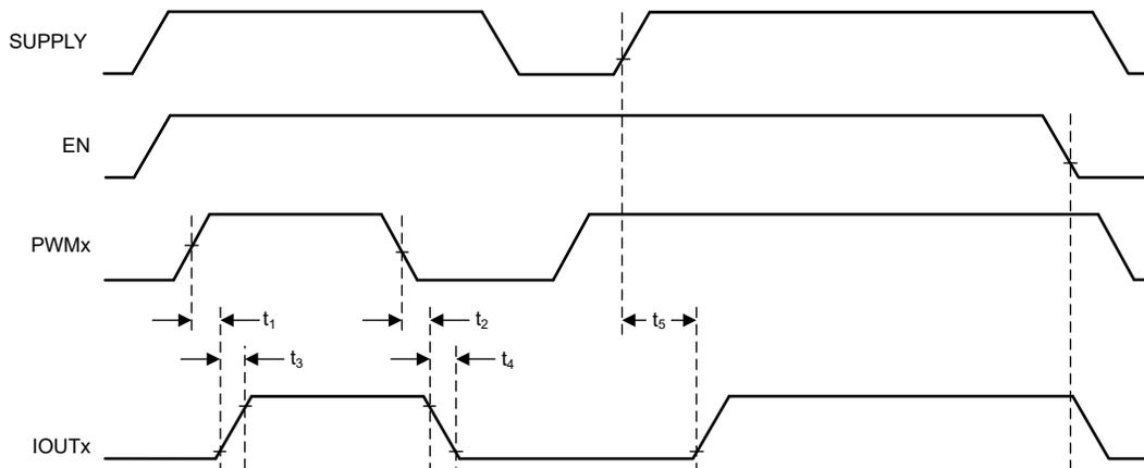
**Figure 6-1. Power-On Sequence and PWM Dimming Timing**
