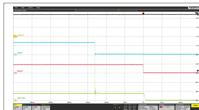
Figure 6-13. LED Short-Circuit Protection
