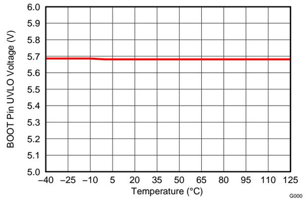
Figure 4. Boot UVLO Threshold vs Junction Temperature
