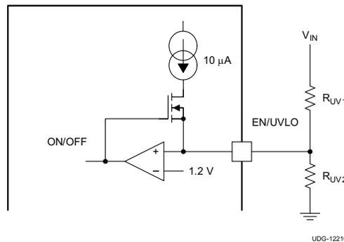
Figure 19. Input UVLO Circuit
