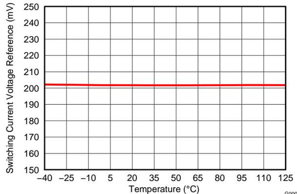
Figure 8. Switching Current Voltage Regulation vs Junction Temperature
