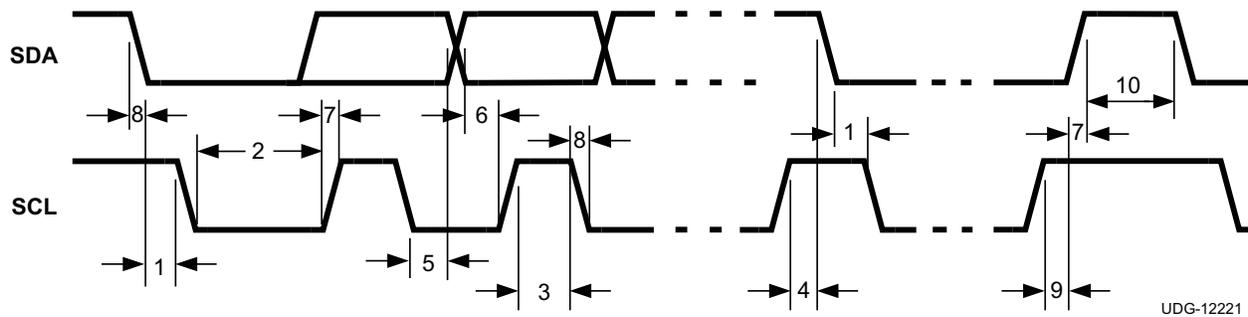
Figure 25. I<sup>2</sup>C Timing Diagram
