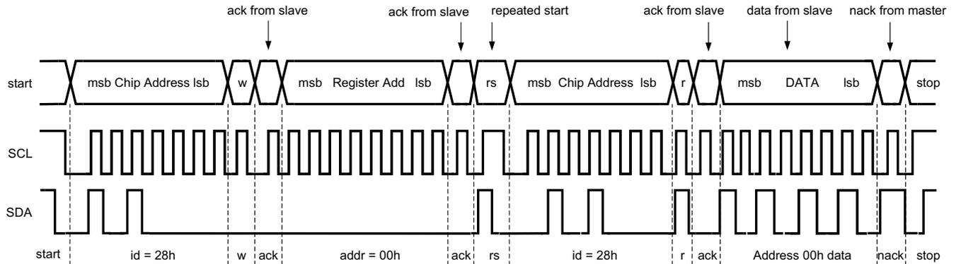
Figure 24. I<sup>2</sup>C Read Cycle
