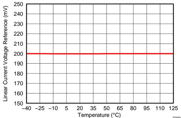
Figure 7. Linear Current Voltage Regulation vs Junction Temperature
