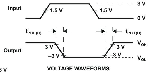
$$SR(tf) = \frac{6\text{ V}}{t_{PHL(D)} \text{ or } t_{PLH(D)}}$$
