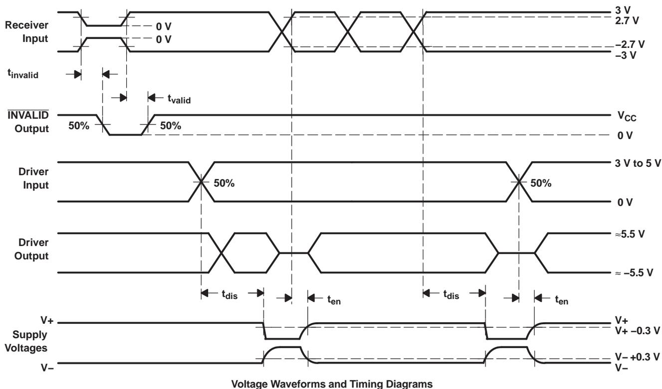
Figure 7.  $\overline{\text{INVALID}}$  Propagation-Delay Times and Supply-Enabling Time
