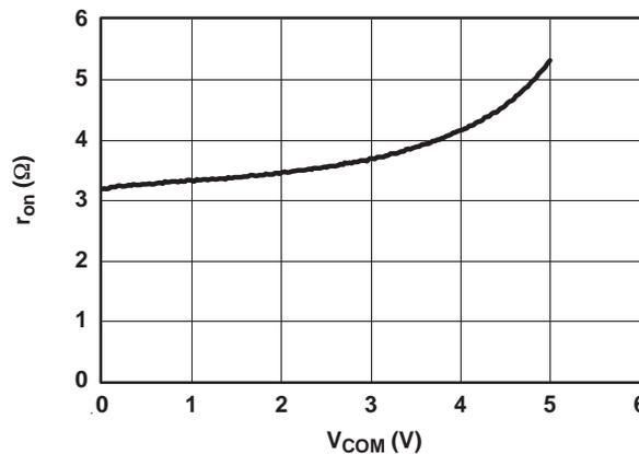
Figure 4. r<sub>on</sub> (Ω) vs V<sub>com</sub> (V)
