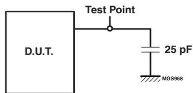
**Figure 6. Load for VM, VP, and RCV**
