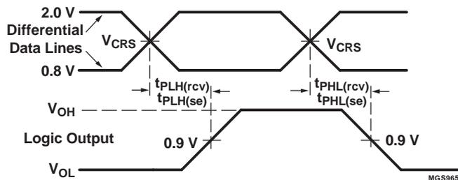
Figure 3. D+, D- to RCV, VP, VM
