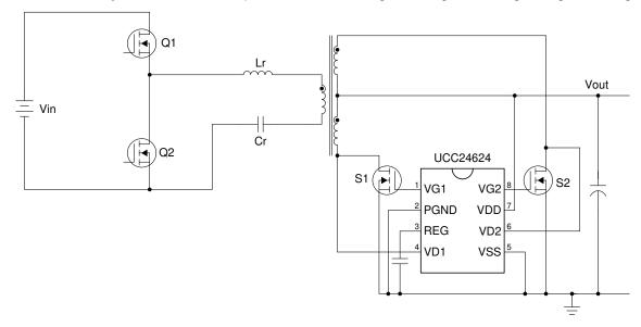
Figure 8-1. UCC24624 Application Diagram in LLC Resonant Converter
