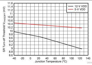
Figure 7-4. SR Turn-off Threshold Voltages vs Temperature
