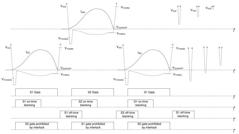
Figure 8-7. Blanking Time and Interlock Logic in UCC24624
