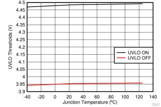
Figure 7-1. UVLO Thresholds vs Temperature
