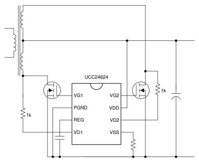
Figure 8-9. UCC24624 configuration with VD resistors
