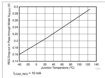
Figure 7-7. REG Dropout in Pass-through Mode vs
