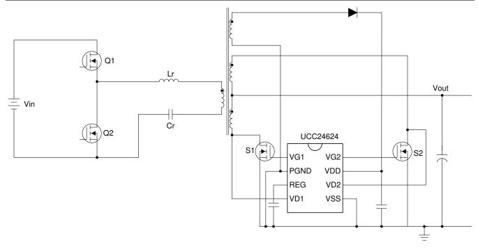
Figure 10-1. Powering UCC24624 Using Auxiliary Winding
