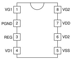
Figure 6-1. D Package 8-Pin SOIC Top View
