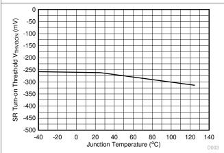
Figure 7-3. SR Turn-on Threshold Voltage vs Temperature
