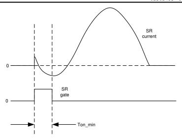
Figure 8-8. SR current with leading edge spike
