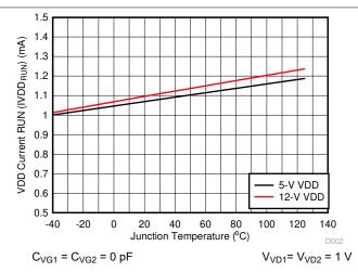
Figure 7-2. Bias Supply Current vs Temperature (No Switching)
