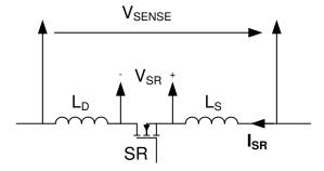
Figure 8-5. SR Controller Sensed Voltage
