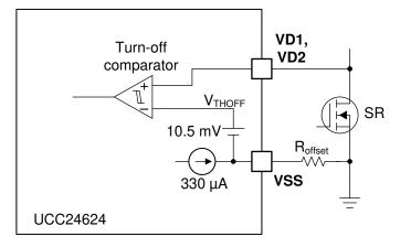
Figure 8-6. Adjustable Turn-off Threshold
