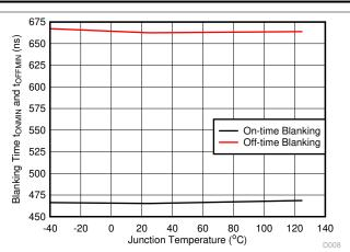
Figure 7-8. Blanking Time vs Temperature
