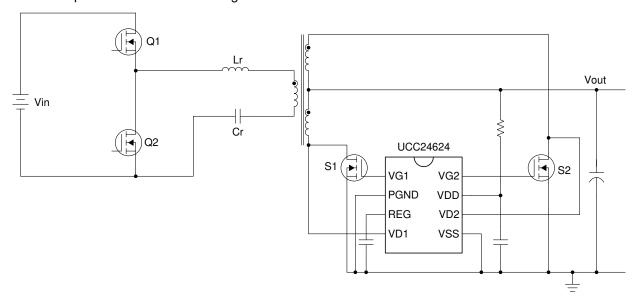
Figure 8-3. UCC24624 Configuration for an Output Voltage Higher Than 24.75 V
