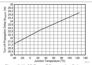
Figure 7-10. SR Turn-off Propagation Delay vs Temperature
