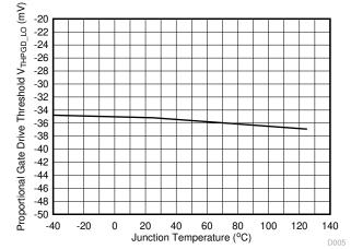
Figure 7-5. Proportional Gate Drive Threshold vs Temperature
