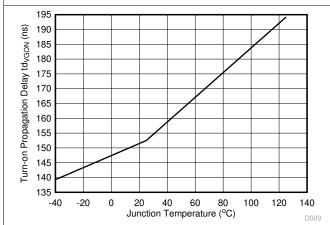
Figure 7-9. SR Turn-on Delay Time vs Temperature
