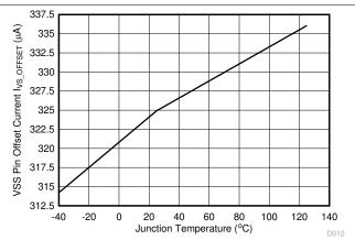
Figure 7-12. VSS Pin Offset Current vs Temperature
