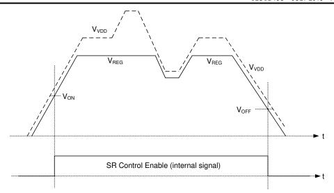
Figure 8-2. Timing diagram for VDD and REG
