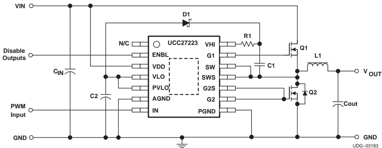
Figure 3. System Application: 8.5-V to 20-V Input
