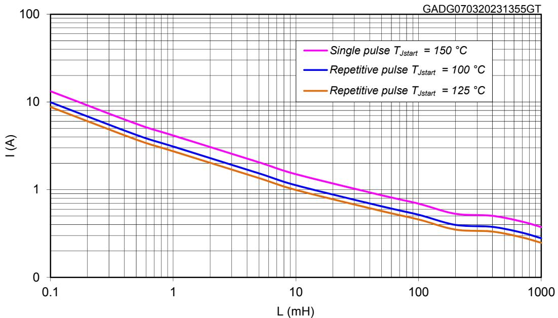
Figure 40. Maximum turn off energy versus inductance
