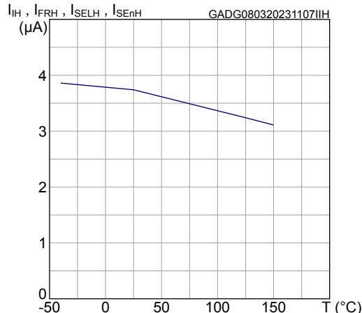
**Figure 18. Low level logic input current**
