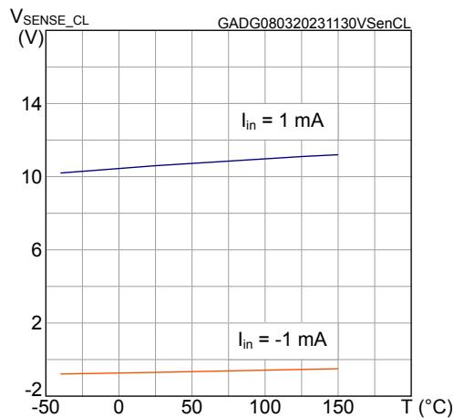
**Figure 31.  $V_{\text{senseh}}$  vs  $T_c$**
