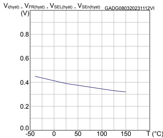
**Figure 20. FaultRST input clamp voltage**
