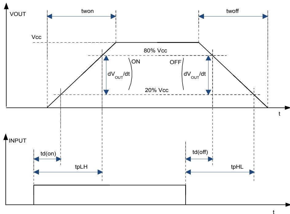
Figure 5. Current sense timings (current sense mode)
