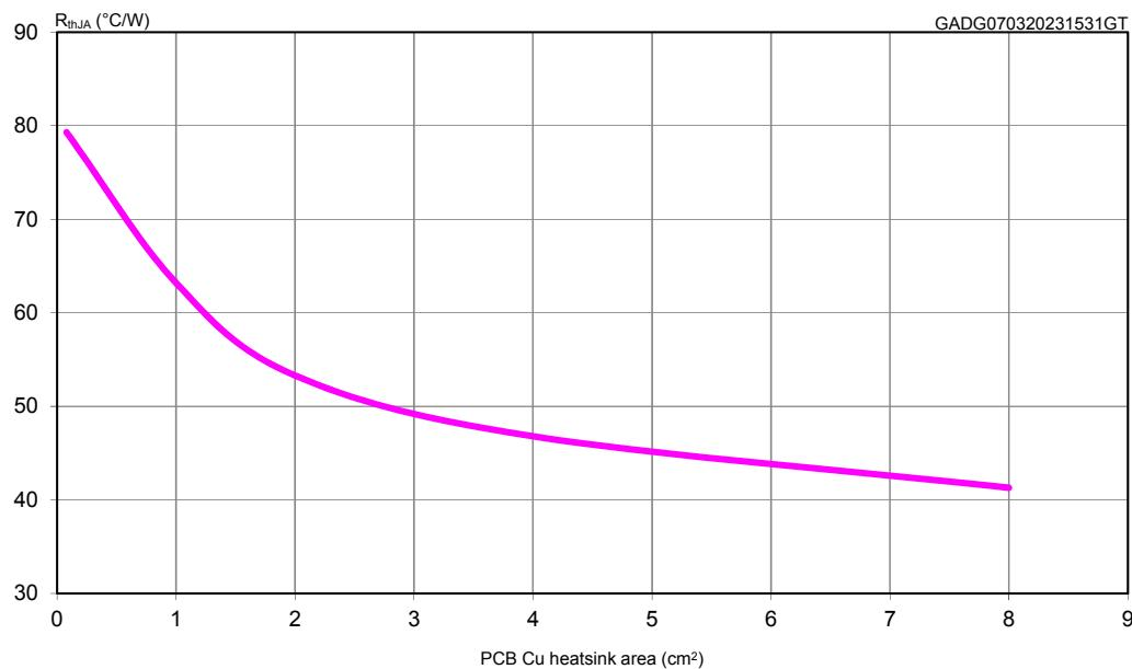
**Figure 44.** PowerSSO-16 thermal impedance junction ambient single pulse (one channel on)
