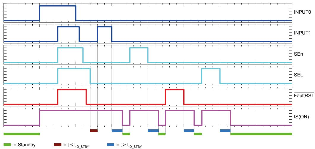
Figure 11. Standby state diagram
