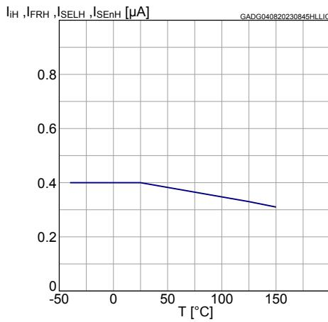
**Figure 18. Low level logic input current**
