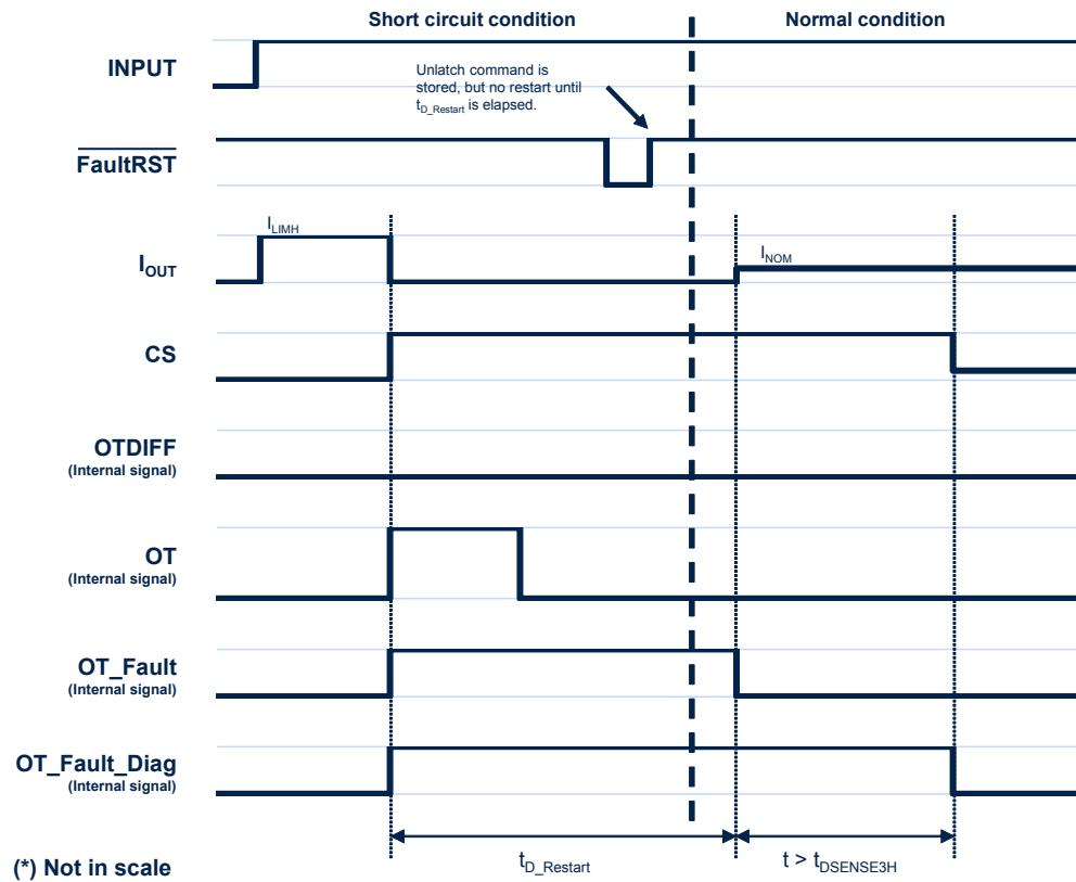
Figure 8. Auto-restart mode - Intermittent short circuit
