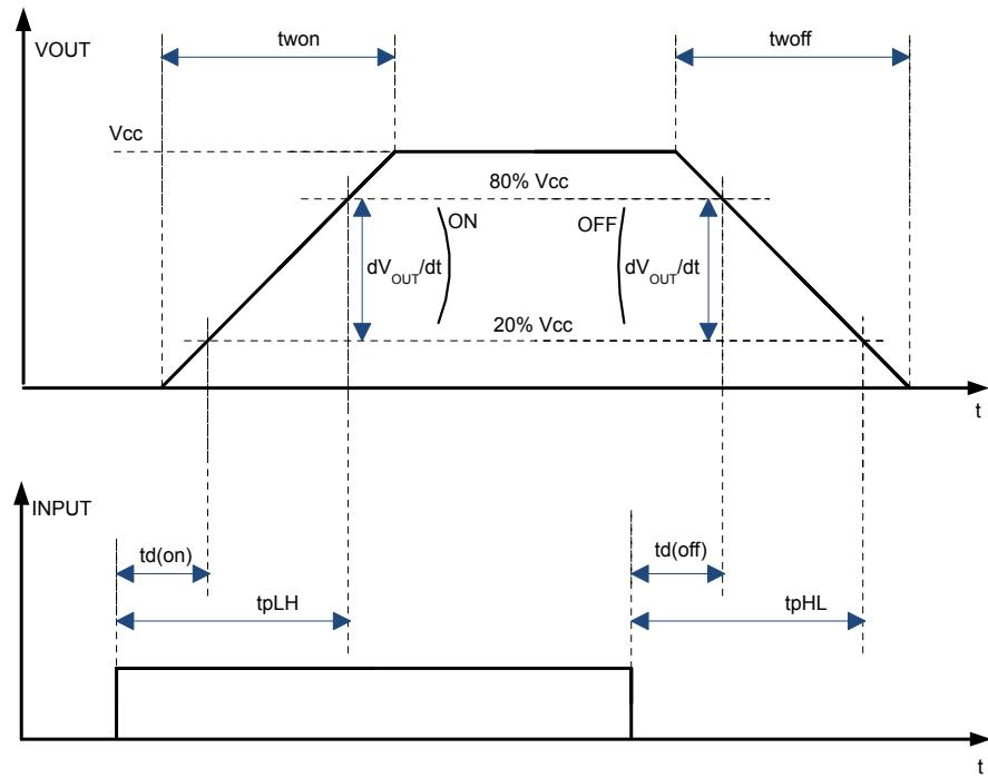
**Figure 5. Current sense timings (current sense mode)**
