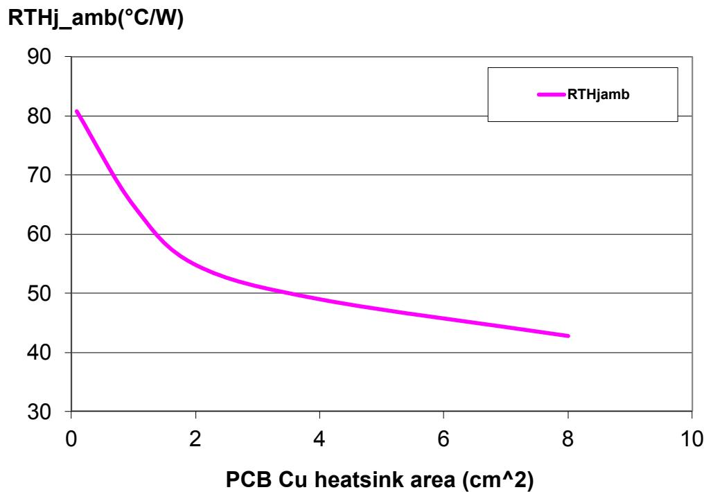
**Figure 44.** PowerSSO-16 thermal impedance junction ambient single pulse (one channel on)
