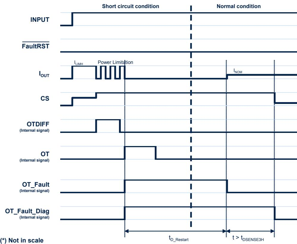
Figure 9. Auto-restart mode - Permanent short circuit
