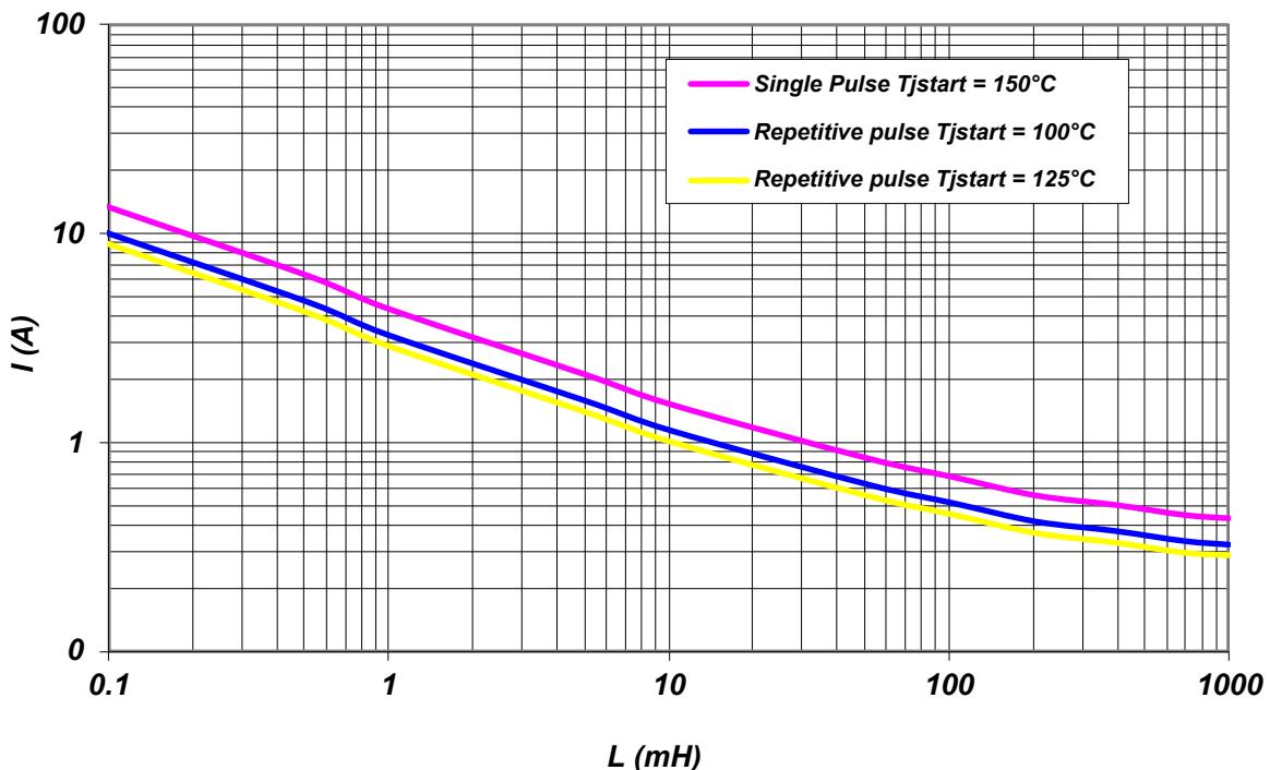
Figure 40. Maximum turn off energy versus inductance
