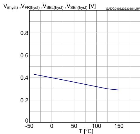
**Figure 20. FaultRST Input clamp voltage**
