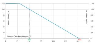
Derating (thermal resist.) UXP°-1000: 9.52 W/K (0.105 K/W)
