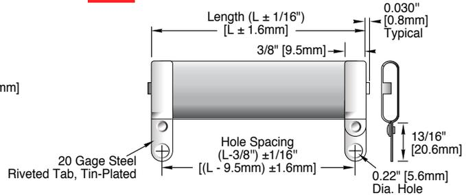
**Fig. 3 With Right Angle Radial Tabs – same direction – (G2)**
