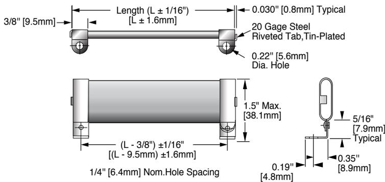
**Fig. 4 With Right Angle Radial Tabs – opposite direction – (G3)**
