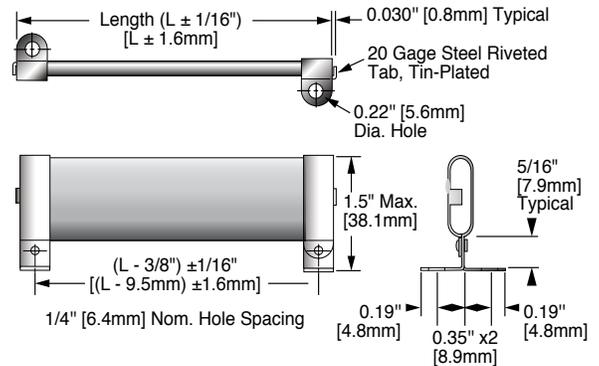
**Fig. 5 With Low Profile Axial Tabs (H1)**
