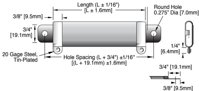
**Fig. 6 With Standoff Axial Tabs (H2)**
