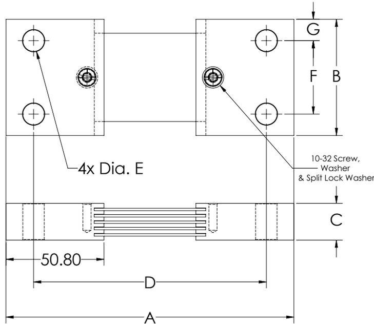
\*Dimension tolerances:  $\pm 0.381\text{mm}$  for hole diameters. All other dimensions have a  $\pm 0.762\text{mm}$  tolerance
