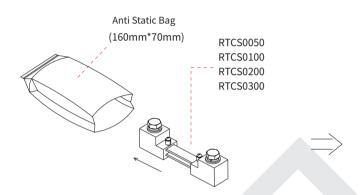
1. Put the product into an anti-static bag and vacuum seal it.
