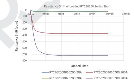
\*Under different heat dissipation conditions and different applied copper bar sizes, there will be some differences in the change of shunt on resistance. The above operating conditions are under normal temperature with 100mm<sup>2</sup> copper wire; For customized test, please contact us to provide detailed operating conditions.
