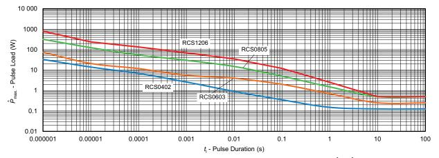
Maximum pulse load, continuous pulses; applicable if  $\overline{P} \leq P$  ( $\vartheta_{amb}$ ) and  $\hat{U} = \hat{U}_{max}$ ; for permissible resistance change equivalent to 8000 h operation
