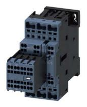
power contactor, AC-3e/AC-3, 38 A, 18.5 kW / 400 V, 3-pole, 220 V AC, 50/60 Hz, auxiliary contacts: 2 NO + 2 NC, spring-loaded terminal, size: S0, removable auxiliary switch
