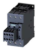
power contactor, AC-3e/AC-3, 51 A, 22 kW / 400 V, 3-pole, 110 V AC, 50/60 Hz, auxiliary contacts: 2 NO + 2 NC, screw terminal, size: S2, removable auxiliary switch
