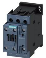
power contactor, AC-3e/AC-3, 32 A, 15 kW / 400 V, 3-pole, 400 V AC, 50 Hz, auxiliary contacts: 1 NO + 1 NC, screw terminal, size: S0
