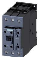
power contactor, AC-3e/AC-3, 51 A, 22 kW / 400 V, 3-pole, 24 V AC, 50 Hz, auxiliary contacts: 1 NO + 1 NC, screw terminal, size: S2, upright mounting position
