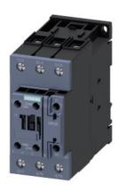
contactor, NEMA version, 25 HP, 460 / 575 V, 3-pole, 20-33 V AC/DC, 50/60 Hz, with integrated varistor, auxiliary contacts: 1 NO + 1 NC, screw terminal, size: S2  $\,$
