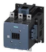
power contactor AC-1 690 A / 690 V / 40  $^\circ$ C 3-pole, Uc: 440-480 V AC(50-60 Hz) / DC drive: conventional auxiliary contacts 2 NO + 2 NC main circuit: busbar control and auxiliary circuit: screw terminal
