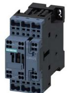
power contactor, AC-3e/AC-3, 17 A, 7.5 kW / 400 V, 3-pole, 110 V DC, auxiliary contacts: 1 NO + 1 NC, spring-loaded terminal, size: S0
