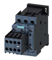
power contactor, AC-3e/AC-3, 32 A, 15 kW / 400 V, 3-pole, 110 V AC, 50 Hz, auxiliary contacts: 2 NO + 2 NC, screw terminal, size: S0, removable auxiliary switch
