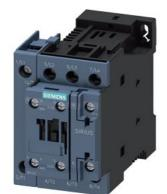
contactor AC-1, 35 A, 400 V / 40  $^{\circ}\text{C},$  4-pole, 220 V DC, auxiliary contacts: 1 NO + 1 NC, screw terminal, size: S0
