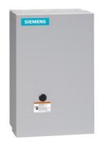
Mechanically held lighting contactor, Contactor amp rating 100A, 0 N.C. / 5 N.O. poles, 208VAC 60HZ coil, Non-combination type, Enclosure NEMA type 1, Indoor general purpose use
