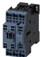
power contactor, AC-3e/AC-3, 25 A, 11 kW / 400 V, 3-pole, 24 V DC, auxiliary contacts: 1 NO + 1 NC, spring-loaded terminal, size: S0, communication-capable
