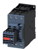
power contactor, AC-3e/AC-3, 80 A, 37 kW / 400 V, 3-pole, 24 V DC, 0.8-1.2\* Us, with integrated varistor, auxiliary contacts: 2 NO + 2 NC, main circuit: screw terminal, control and auxiliary circuit: spring-loaded terminal, size: S2, suitable for PLC outputs, captive auxiliary switch
