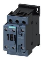
power contactor, AC-3e/AC-3, 32 A, 15 kW / 400 V, 3-pole, 400 V AC, 50 Hz / 400-440 V, 60 Hz, auxiliary contacts: 1 NO + 1 NC, screw terminal, size: S0
