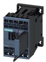
traction contactor, AC-3e/AC-3, 16 A, 7.5 kW / 400 V, 3-pole, 110 V DC, 0.7-1.25\* Us, with integrated varistor, auxiliary contacts: 1 NC, spring-loaded terminal, size: S00, with plugged on series resistor
