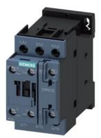
contactor, NEMA version, 10 hp, 460 / 575 V, 3-pole, 600 V AC, 60 Hz, auxiliary contacts: 1 NO + 1 NC, screw terminal, size: S0
