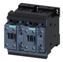
reversing contactor assembly, AC-3e/AC-3, 9 A, 4 kW / 400 V, 3-pole, 24 V DC, screw terminal, electrical and mechanical interlock, auxiliary contacts: 2 x 1 NO
