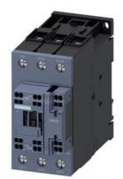
power contactor, AC-3e/AC-3, 80 A, 37 kW / 400 V, 3-pole, 20-33 V AC/DC, 50/60 Hz, with integrated varistor, auxiliary contacts: 1 NO + 1 NC, main circuit: screw terminal, control and auxiliary circuit: spring-loaded terminal, size: S2,
