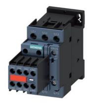
power contactor, AC-3e/AC-3, 38 A, 18.5 kW / 400 V, 3-pole, 230 V AC, 50/60 Hz, auxiliary contacts: 2 NO + 2 NC, screw terminal, size: S0, captive auxiliary switch, no surge suppressor retrofittable
