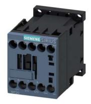
power contactor, AC-3e/AC-3, 16 A, 7.5 kW / 400 V, 3-pole, 80 V DC, auxiliary contacts: 1 NC, screw terminal, size: S00  $\,$
