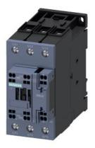
power contactor, AC-3e/AC-3, 65 A, 30 kW / 400 V, 3-pole, 175-280 V AC/DC, 50/60 Hz, with integrated varistor, auxiliary contacts: 1 NO + 1 NC, main circuit: screw terminal, control and auxiliary circuit: spring-loaded terminal, size: S2,
