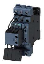
capacitor contactor, AC-6b 33 kVAr, / 400 V, 3-pole, 24 V AC, 50 Hz, auxiliary contacts: 1 NO + 2 NC, screw terminal, size: S0  $\,$
