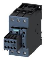
power contactor, AC-3e/AC-3, 41 A, 18.5 kW / 400 V, 3-pole, 24 V DC, 0.8-1.2\* Us, with integrated varistor, auxiliary contacts: 2 NO + 2 NC, screw terminal, size: S2, suitable for PLC outputs, removable auxiliary switch
