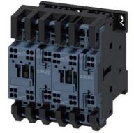
reversing contactor assembly, AC-3e/AC-3, 25 A, 11 kW / 400 V, 3-pole, 230 V AC, 50/60 Hz, spring-loaded terminal, electrical and mechanical interlock, auxiliary contacts:  $2 \times 1 \text{ NO}$
