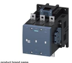
vacuum contactor AC-3e/AC-3 400 A, 200 kW / 400 V, 3-pole, Uc: 220-240 V AC(50-60 Hz) / DC drive: conventional auxiliary contacts 2 NO + 2 NC main circuit: busbar control and auxiliary circuit: screw terminal
