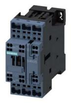
power contactor, AC-3e/AC-3, 25 A, 11 kW / 400 V, 3-pole, 125 V DC, 0.7-1.25  $^{\star}$  Us, with plugged-in varistor, auxiliary contacts: 1 NO + 1 NC, spring-loaded terminal, size: S0, suitable for PLC outputs, not expandable with auxiliary switch
